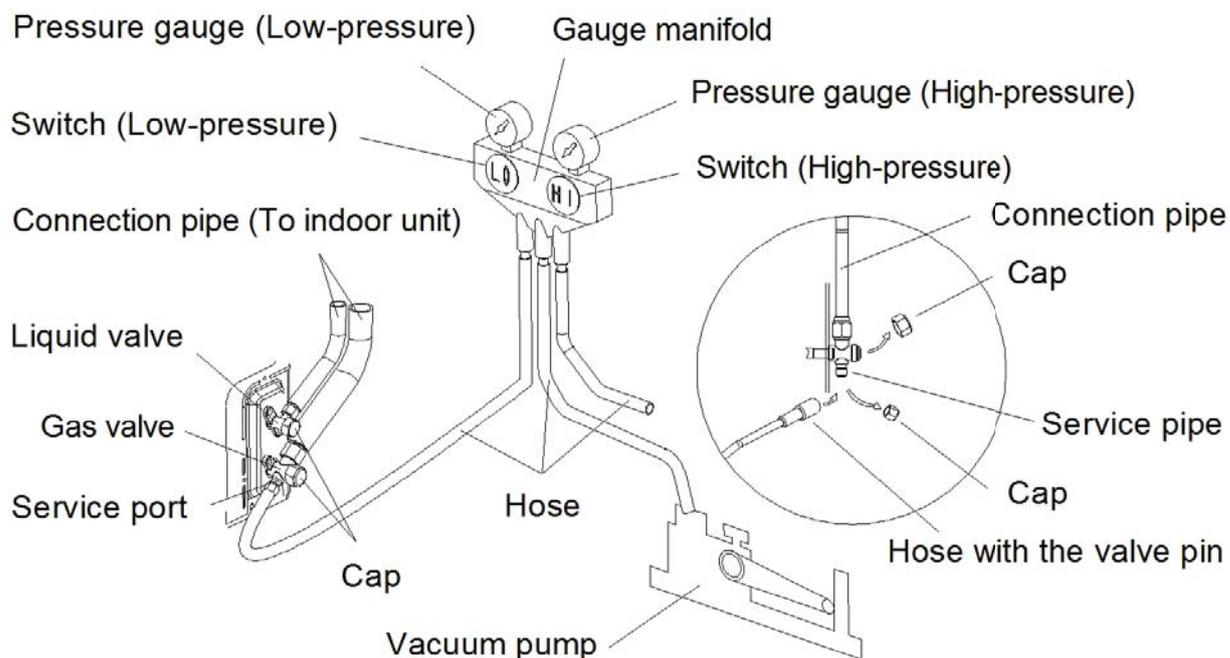
**NOTICE** For large-size units, there are maintenance ports for liquid valve and gas valve. During evacuation, you may connect the two hoses of the branch valve assembly to the maintenance ports to speed up the evacuation.
