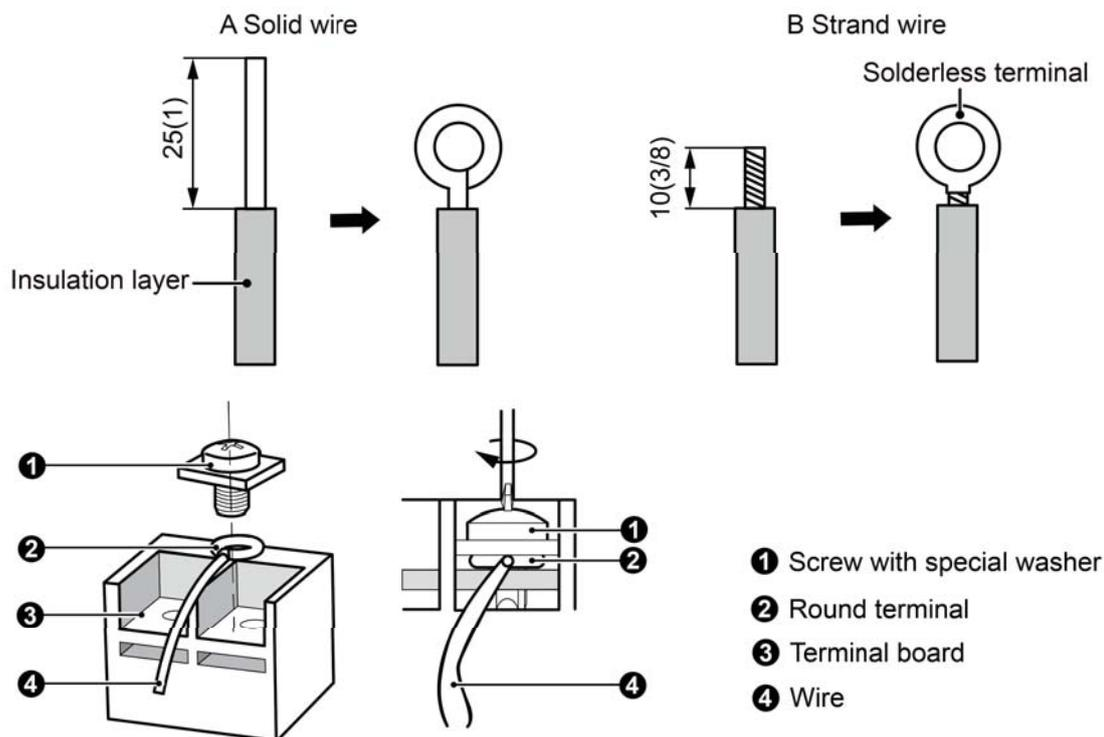
(3) How to connect the the temperature controller wire and power cord.
