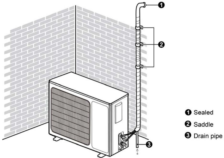
(2) If the outdoor unit is above the indoor unit, arrange the pipeline according to the following diagram.
